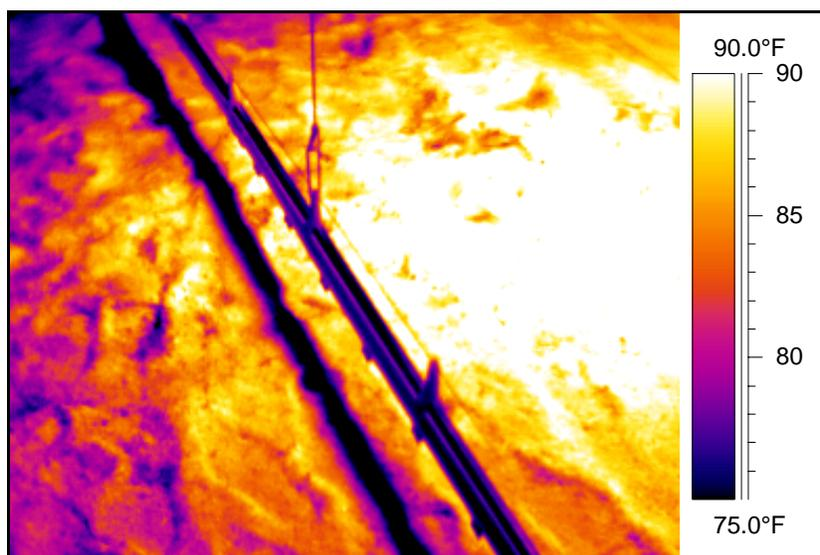
Figure 16. Shadow cast by drinker line.
