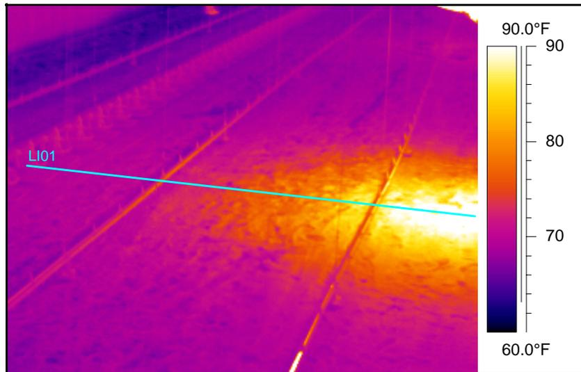
Figure 2. Single radiant brooder is 70°F house.
