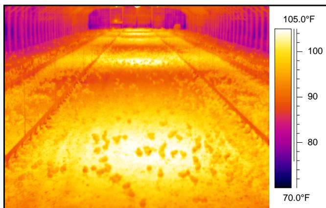
Figure 14. Side wall in house with radiant tube brooders      Figure 15. Center of house with radiant tube brooders
