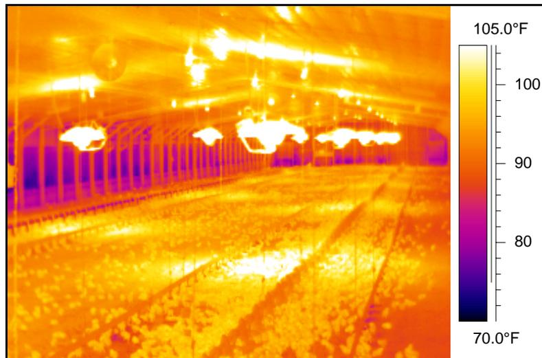
Figure 1. Thermal image of brooding area with radiant brooders.
