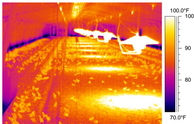
Figure 13. Center house floor temperatures.
