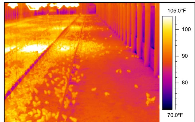
Figure 7. Thermal image near side wall with chicks present.
